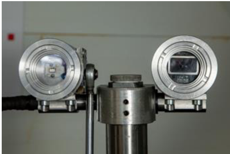
Video surveillance and searchlight system of the robot
