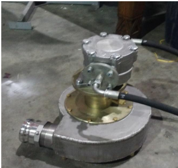
Booster (centrifugal) pump of the robot for low viscosity sludge (capacity up to 60 cbm of oil sludge per hour )
